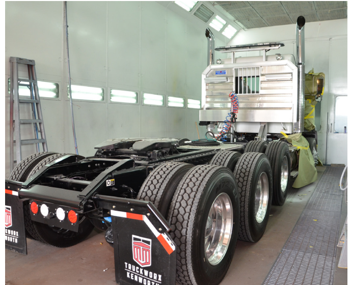
Seventy-foot downdrafted heated paint booth at Truckworx Body Shop
